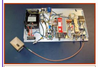
A **10 GHz** Transverter and horn antenna made from "just parts" by Randy NR6CA. Photo courtesy Mike WB2RVX
